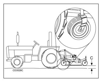
Figure 8. Front Caster Wheel Interference Check
